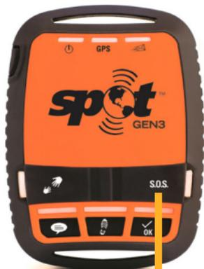
Open flap and press and hold the SOS button until SOS indicator flashes to raise a test alarm
