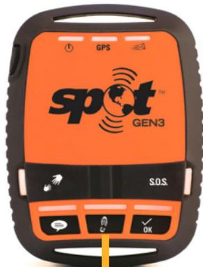
Press and hold automatic position button until indicator flashes to enable tracking
